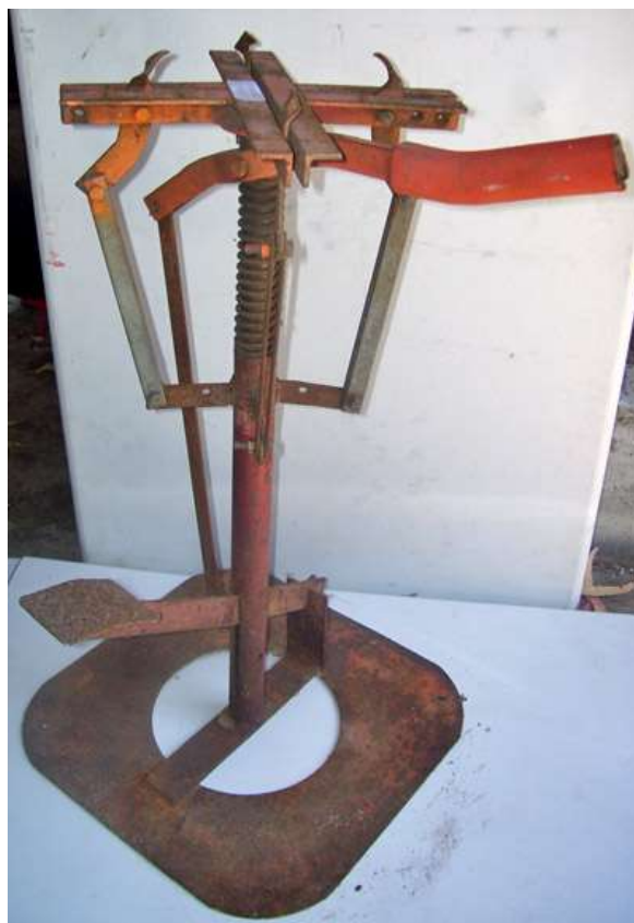
From top left, clockwise: Can cutter. Used to cut open metal potting cans. Not used for years since industry changed to plastic cans.
